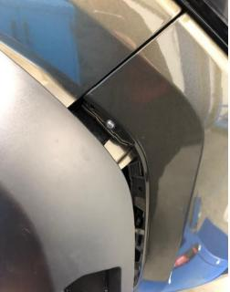
7. Gently peel back flare unclipping it from inside the bumper, revealing a silver screw. Remove and retain screw for re-fitment.
