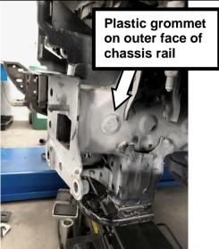
29. Remove the three forwardmost plastic gromets on the chassis rails. One on chassis rail outer face, one on inner face and one on lower face.
