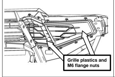
90. Fit grille plastics to bar using twenty M6 flange nuts. Torque to spec.
