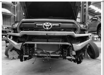
41. Fit bar to vehicle using lifting aid such as an elevating trolley.
