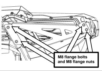
91. Fit wing braces to bar using eight M8 flange bolts and eight M8 flange nuts. Torque to spec.
