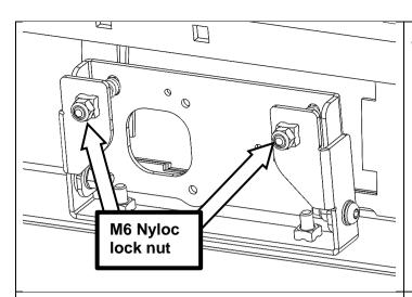
88. Lock the radar adjustment in position with two M6 Nyloc nuts tightened against the radar bracket as shown. Hold adjustment bolts in place when tightening. Torque to spec.
