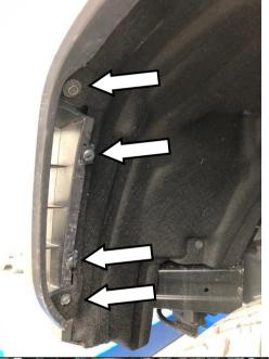
3. Remove the clips & screws holding the front half of the wheel arch liners.
