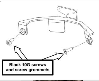
28. Secure trimmed bumper to bumper retention brackets using two 10G black screws and two screw grommets through the bumper. Right hand side shown.
