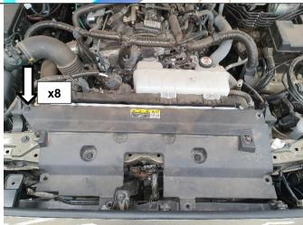
4. Open the bonnet and remove all scrivets (8) retaining plastic cover. Set aside scrivets removed for re-use later on.
