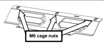
95. Fit three M6 cage nuts to stone tray.
