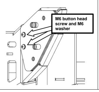
38. Install mount shims to the mount using two M6x20 button head bolts with M6 washers. Torque to spec.
