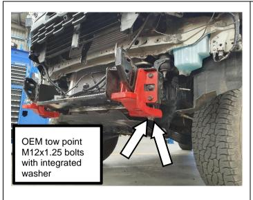
36. Install two OEM tow point M12x1.25 bolts with integrated washer removed in step 2. Left hand side shown. Leave fasteners loose.
