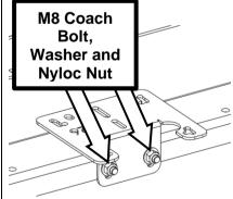
Fit the winch to the cradle and the hawse/fairlead to the bash plate. Skip to step 70.
