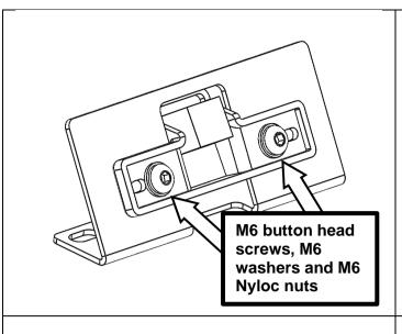
39. Fit camera to bracket using two M6 button head screws, four M6 washers and two M6 Nyloc nuts. Tighten until firm taking care to not damage plastic camera bracket.
