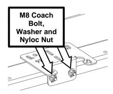
Fit the winch to the cradle and the hawse/fairlead to the bash plate. Skip to step 70.
