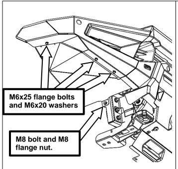
94. Secure the RH wing under panel using three M6 flange bolts, three M6x20 washers, an M8 bolt and an M8 flange nut. Torque to spec.
