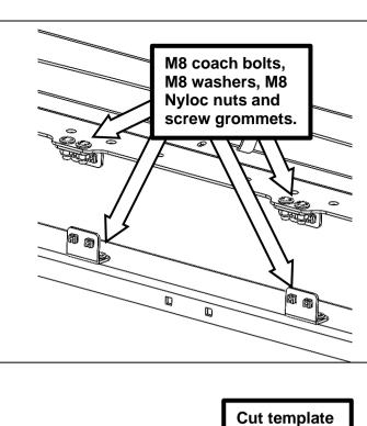
64. Install four grille retention brackets using two M8 coach bolts, two M8 washers and two M8 Nyloc nuts **per bracket**, orientation as shown. Torque to spec.
