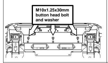
81. Fit three M10x1.5x30 button head screws, three M10 washers and three 10 mm packers (single hole) to secure the bottom of the bash plate to the winch cradle. Leave fasteners loose.
