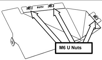
92. Fit M6 U nuts to both under panels as shown, six total.
