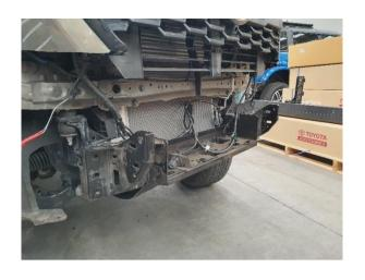
33. Sit the winch cradle in place on the end of the chassis rails as shown. Use studs on front of chassis rail to help location.
