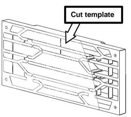
66. Cut out and apply grille template to rear face of grille, aligning the grille pattern printed on the template. Mark the cut line on the back side of the grille.
