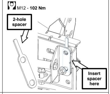
M12x1.25x40mm flange bolt, M12 washer and flange nut
