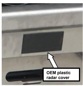
89. Remove OEM plastic radar cover from OEM bumper and clip into aperture in bash plate. Make sure clips fully engage and cover is in the same orientation as fitted to the OEM bumper for a secure fit ("DO NOT PAINT" text right way up).
