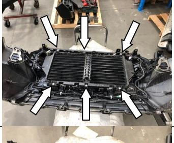
14. Remove six M6 bolts holding the OEM air shutter assembly.
