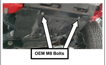
96. Remove front two bolts from OEM underpanel. Fit Zenith stone tray on top, securing with same OEM M8 bolts. Secure with further three M6 button head screws and three M6 washers through the bash plate. Torque to spec.
