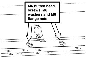
40. Fit bracket with camera to the bar using two M6 button head screws, two M6 washers and two M6 flange nuts. Torque to spec.
