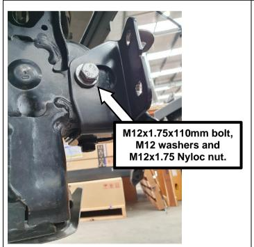
Install one M12x1.75x110 bolt, two M12 washers and a M12 Nyloc nut to each crush tube (two crush tubes). Leave fasteners finger tight.
