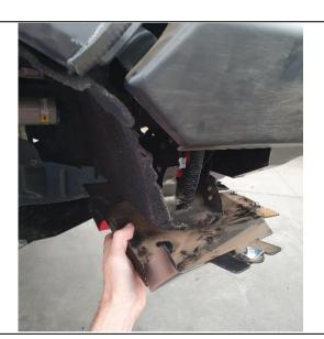
93. Place the RH under panel in position while tucking the wheel liner in place.
