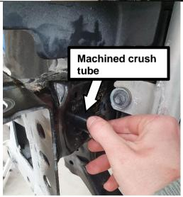
30. Identify and fit a machined crush tube into each chassis rail (RHS and LHS) from the inside.
