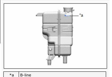
(d) Squeeze the No. 1 radiator hose and No. 2 radiator hose several times by hand, and then check the level of the engine coolant.
