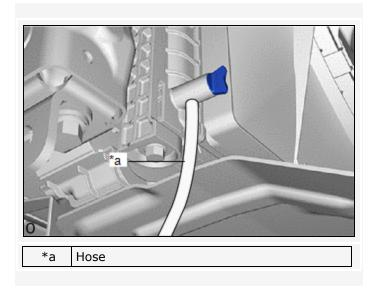
(b) Remove interface degass plug.
