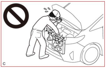
engine compartment with the engine running.
