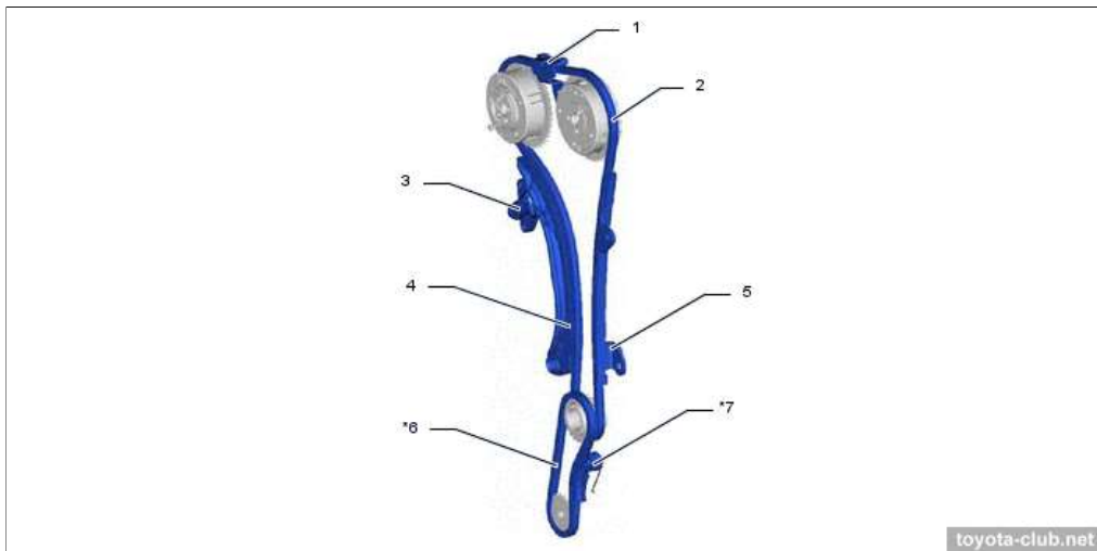
1 - chain vibration damper #2, 2 - timing chain, 3 - chain tensioner 1, 4 - chain tensioner slipper, 5 - chain vibration damper 1, 6 - oil pump drive chain, 7 - chain tensioner plate
